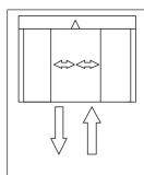
Both presence detection sensors, 1 x interior and 1 x exterior, are activated and open the sliding doors when presence is detected.
