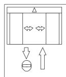
Only the interior presence detection sensor is activated and opens the sliding door when presence is detected.
