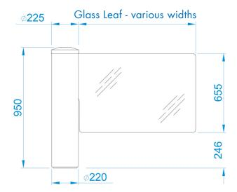
Product delivered in a kit form i.e. Leaves and Rotor and may require lifting equipment.
